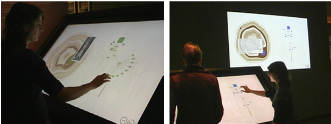
Figure 5.2: Physical setup of EMDialog: tilted direct-touch display (left) and wall projection(right).
